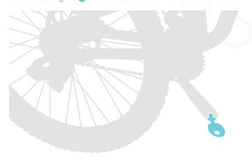
With speedplay pedals (www.speedplay.com) you will want the spindle of the pedal to rest directly on the  $\bigcirc$  Crank Holder at the base of the V-groove.
